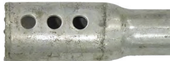
Figure 1.13 Upset coupler with oversized, closely spaced bolt holes
