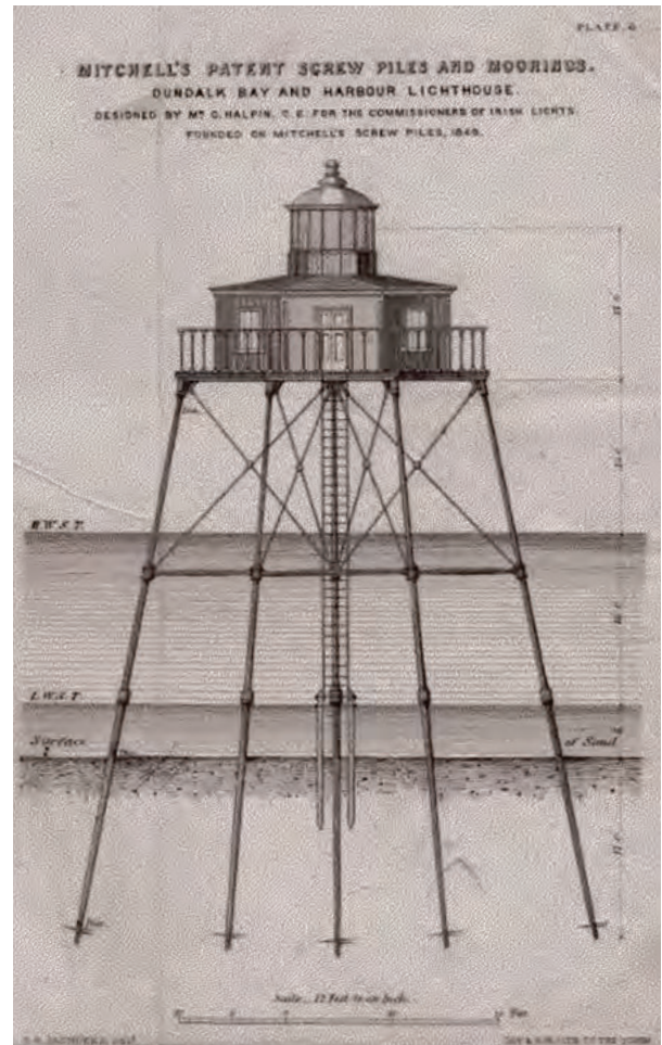
Figure 1.2 Early patent of screw (helical) piles
