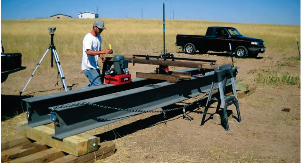
Figure 1.56 Tension load test
