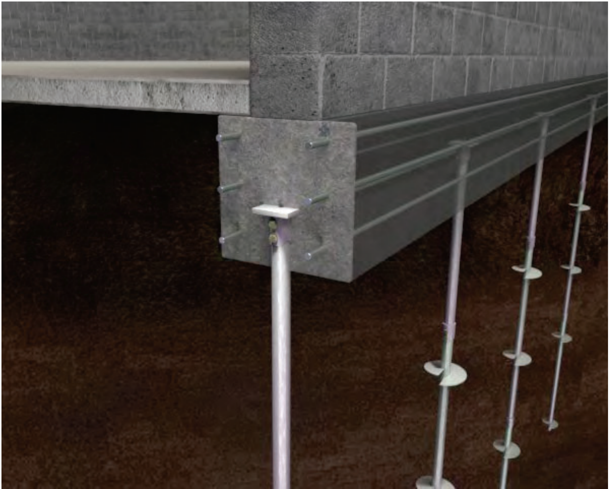
Figure 1.24 Rendering of new construction helical piles cast into a structural grade beam
