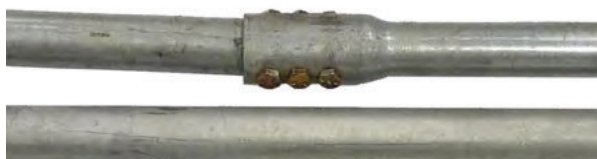
Figure 1.15 Competitor upset coupler variance from straightness
