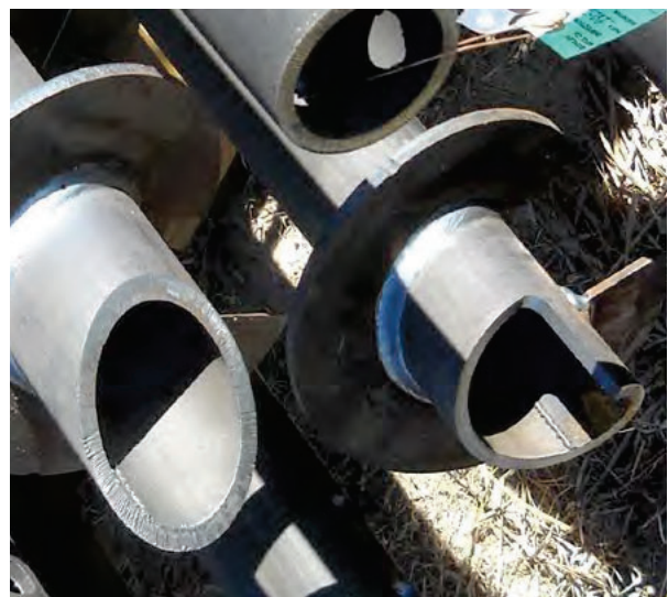
Figure 1.9 45-degree, bevel-cut tip and spiral-cut tip geometry
