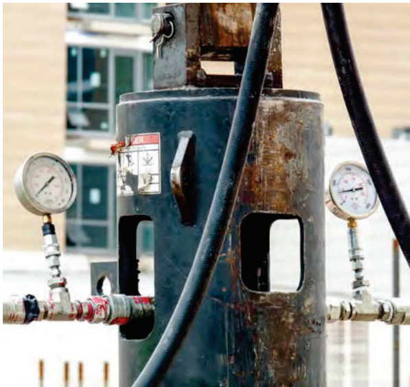
Figure 1.70 Dual pressure gauges
