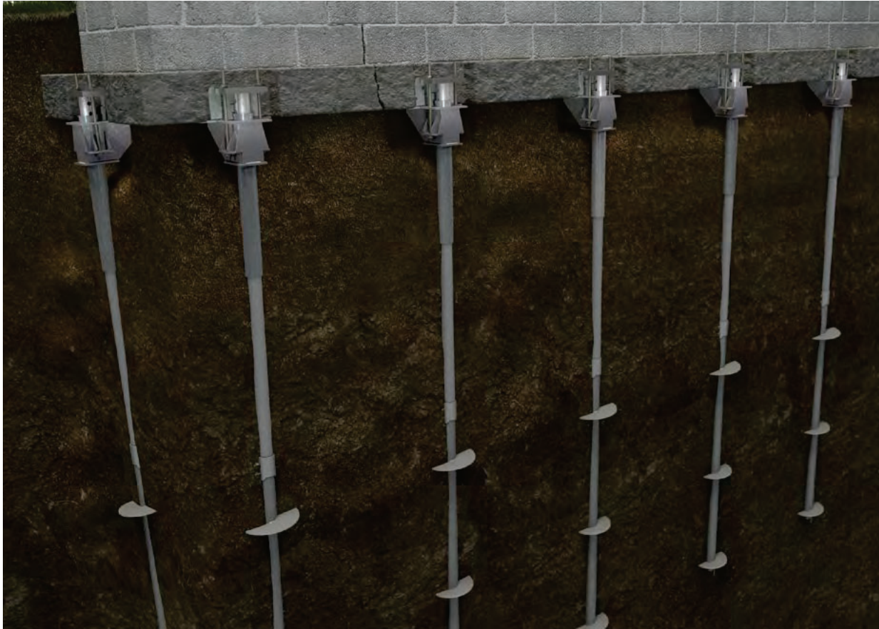
Figure 1.26 Rendering of retrofit helical piers
